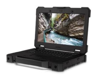
**The Latitude 14 Rugged Extreme laptop** sets a new standard for the most extreme rugged devices. Its armored frame is built around a rigid magnesium alloy backbone. It also features exclusive shockDabsorbent ultraDpolymer materials. This allows the laptop to take serious abuse with ease. It's equipped with a glare-free resistive touch screen, which means it can be operated with heavy work gloves in direct sunlight.
