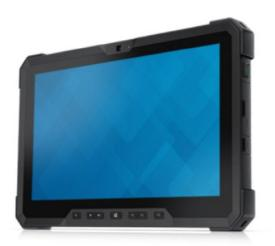
**The Latitude 12 Rugged Tablet** has been designed to operate in extreme conditions. Its 11.6-inch display is Gorilla Glass-protected, and allows you to see in direct sunlight. The multi-touch display can be operated with thick gloves, and even responds in rain.
